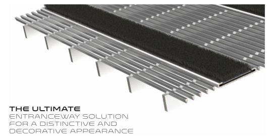
The grating is a combination of stainless steel surface wires, which create a cleaning/scraping process, along with carpet inserts spaced every 4" on center, to clean and dry shoe traffic.
